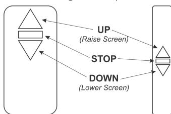
LOWER the screen and STOP the screen at the bottom of the wood rail moulding on the wall. This is an approximate location for the image fitting perfectly on the screen. You can make adjustments as required.
